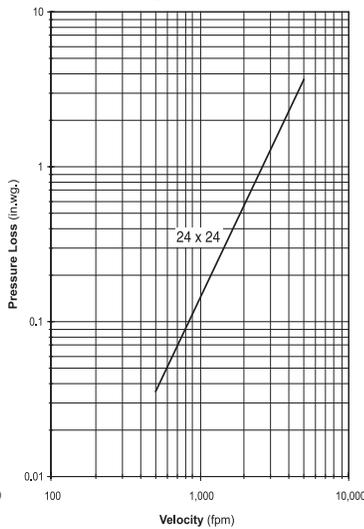
Pressure drop testing was performed in accordance with AMCA Standard 500-D using the three configurations shown. All data has been corrected to represent air density of 0.075 lb/ft. Actual pressure drop in any ducted HVAC system is a combination of many elements. This information, along with analysis of other system influences, should be used to estimate actual pressure losses for a damper installed in a given HVAC system.
