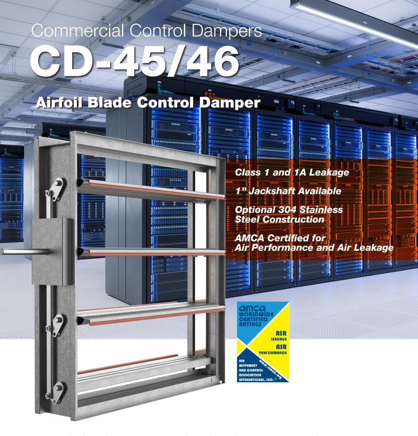
Pottorff's **CD-45** (parallel-blade action) and **CD-46** (opposed-blade action) control dampers feature high-performing airfoil blades and a rugged hat channel frame to provide exceptional air control in medium to high pressure and velocity applications. They are a great solution for regulating airflow and reducing energy consumption for data centers, warehouses and distribution centers.
