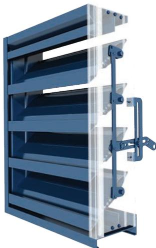
*The EXA-645 design features stationary drainable louver blades to protect against water penetration and an integral airfoil blade control damper to allow positive shut-off of air intake and exhaust openings.*
