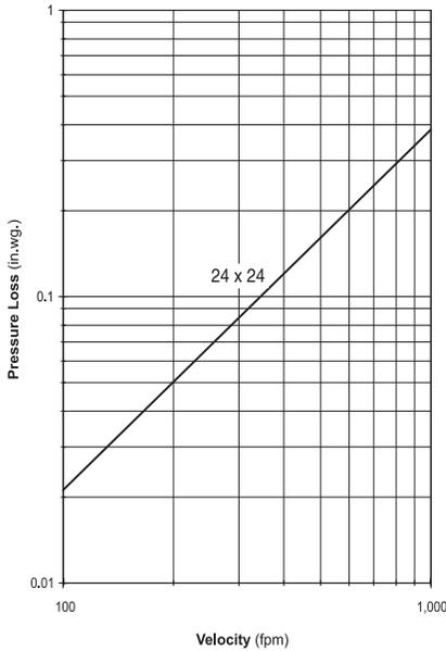
Pressure drop testing was performed in accordance with AMCA Standard 500-D using Figure 5.5 — Plenum Mount. All data has been corrected to represent air density of 0.075 lb/ft. Actual pressure drop in any ducted HVAC system is a combination of many elements. This information, along with analysis of other system influences, should be used to estimate actual pressure losses for a damper installed in a given HVAC system.
